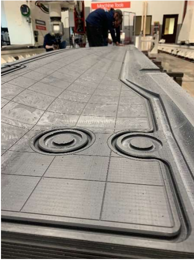
Tool surface after machining is complete, prior to sealing.
