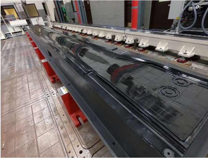
Finished machined and vacuum sealed tool.
